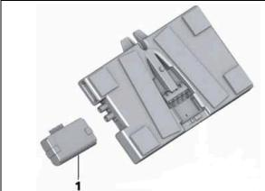
For the eligible vehicles, BMW of North America, LLC (BMW NA) is extending the coverage for the vehicle's **Telematics Control Unit's (TCU) Emergency (Backup) Battery (Item # 1)** to:
