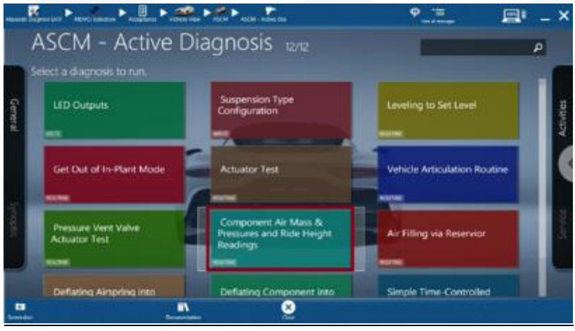
Figure 1: air suspension system pressure reading with the Active Diagnosis of the ASCM ECU.
