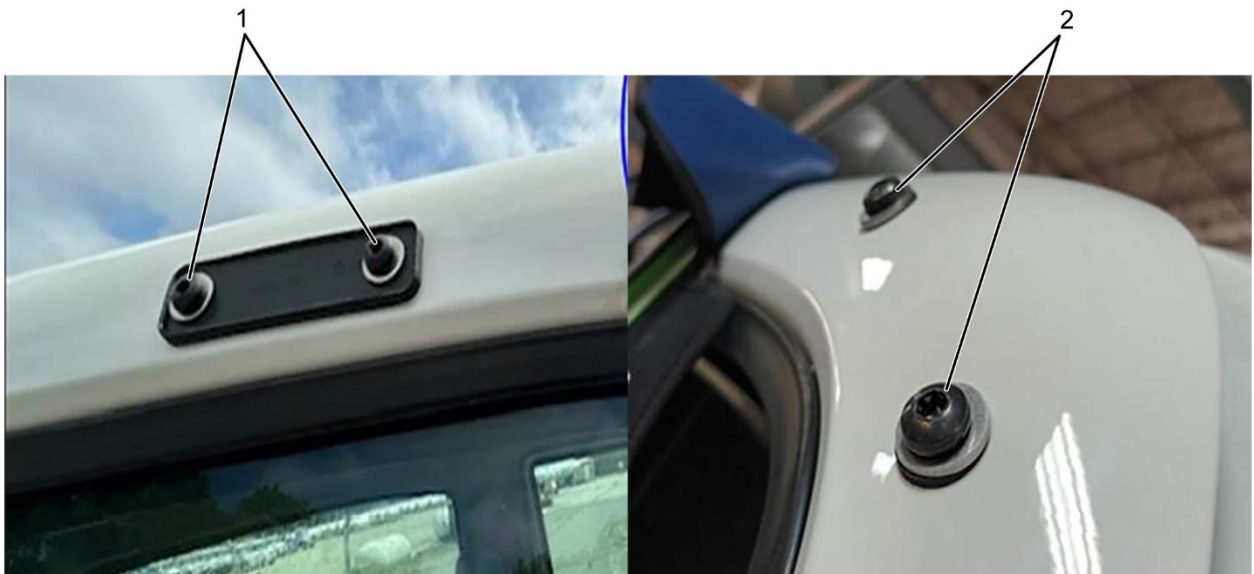
Figure 2. C-Loop Mirror hardware properly installed
