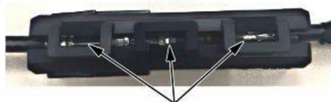
Exposed slice visible.
