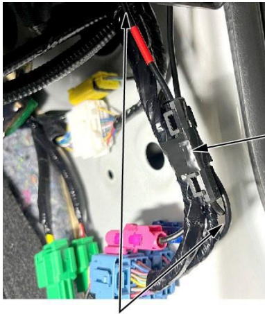
Attach the FAKRA service cable and splice box to the appropriate component harness with tape to prevent any rattles.
