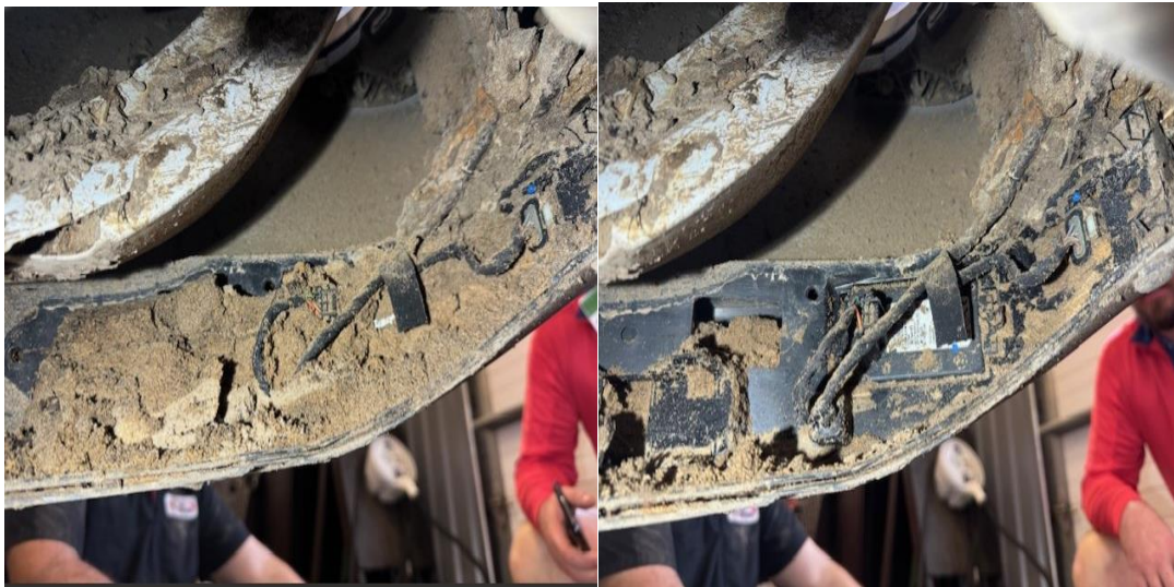
Left Rear Radar Module Shield Removed Showing Dirt Packing Condition.
