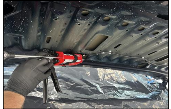
Figure 6. Nozzle Inserted at an Angle
