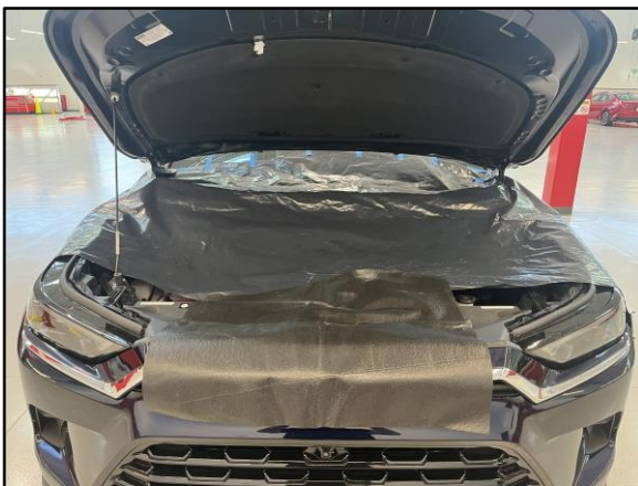
Figure 2. Protected Engine Bay
