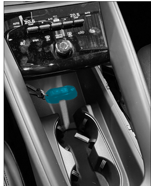
Original handheld transmitter in emergency start tray
