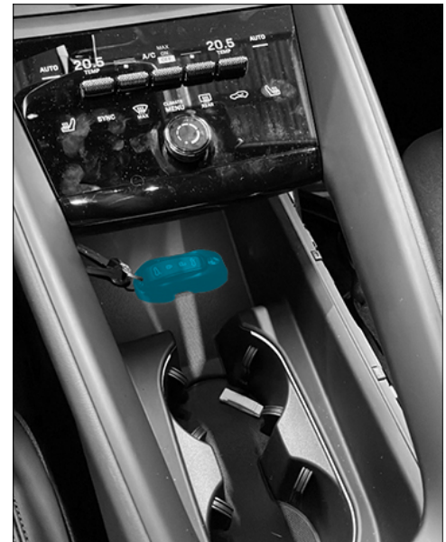
Original handheld transmitter in emergency start tray
