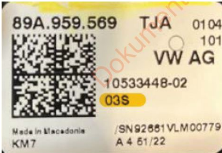
Figure 1. Production label on interior light module with generation 03S.
