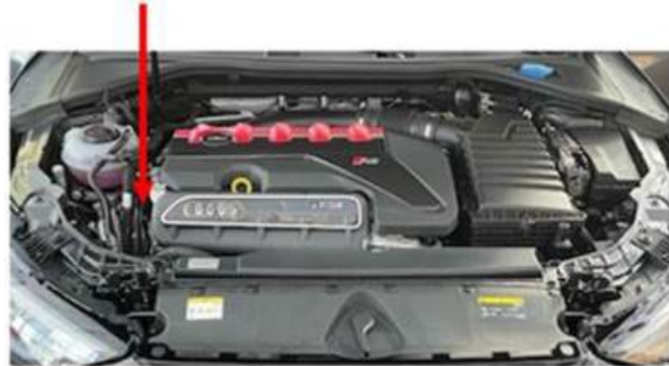
Figure 1. Area of the engine compartment to inspect refrigerant line contact.
