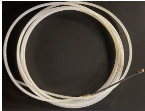
Figure 6. Cleaning tool SET6620 (formerly VAS6620).
