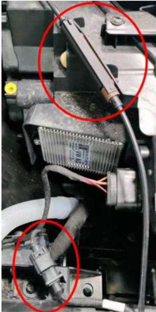
Figure 5. Disconnect hood switch and hood cable.
