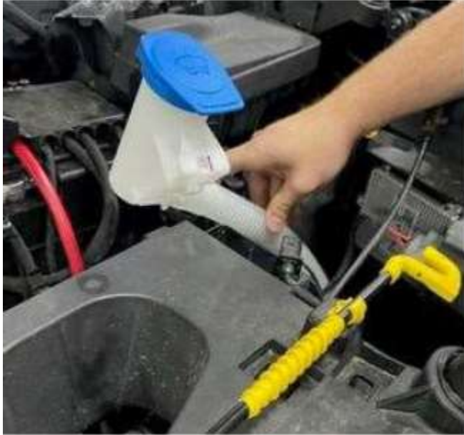
Figure 6. Set aside washer solvent filler neck.
