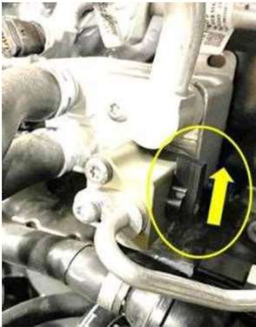
Figure 16. Installation of A/C Line connection block adaptor VAS 6338/80.
