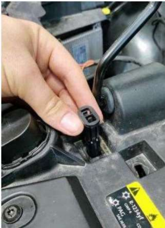
Figure 7. Remove radiator module bracket.
