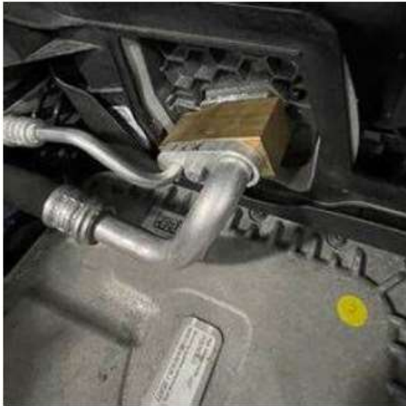
Figure 15. Installation of front expansion valve bypass adaptor VAS 6338/38.
