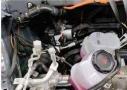
Figure 4. Coolant reservoir set aside.
