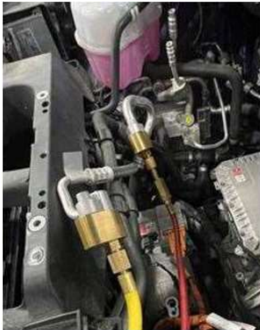
Figure 18. Installation of VAS 6338/3 and 6338/12.
