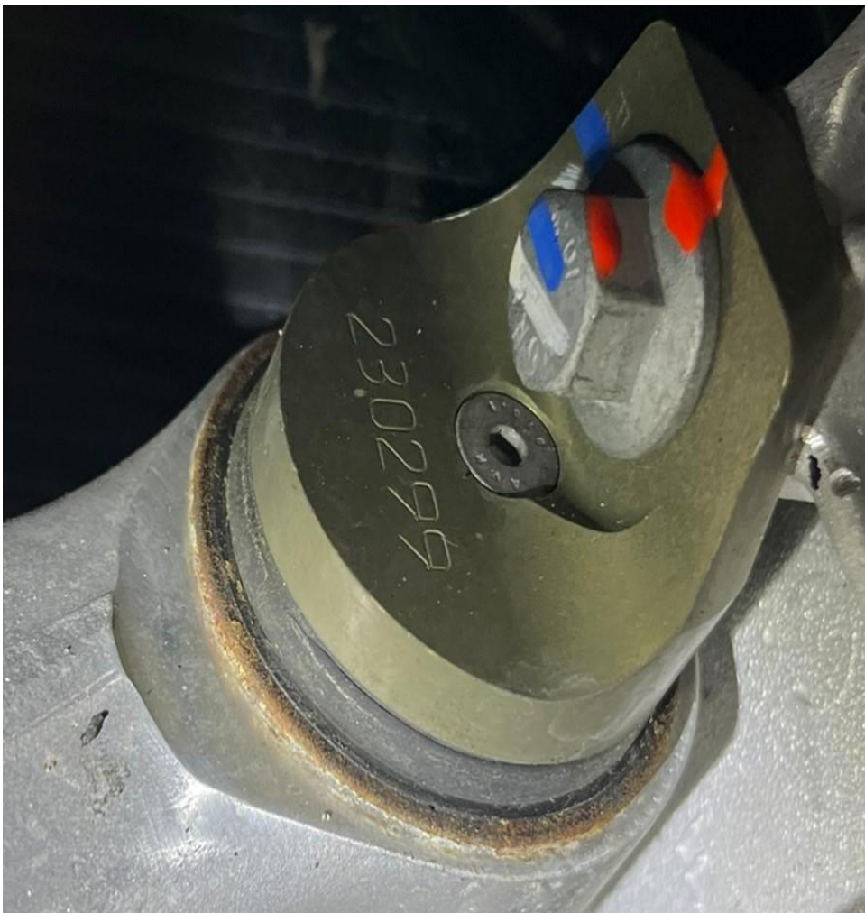
(Example 2 - Bush outer metal dirt accumulation.)
