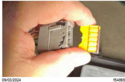
Fig. 87, TPMS Connector With Orange Terminal Retention Lock Removed
