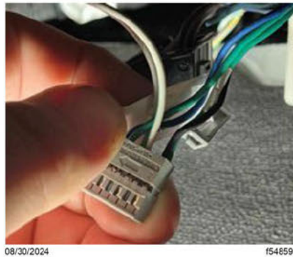
Fig. 23, Gray Connector Removed from Main CGW Connector Housing
