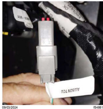
Fig. 46, End Cap Installed on Engine Harness Overlay Connector Labeled 'ALLISON TCU'
