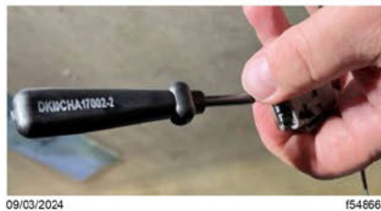
Fig. 89, Removing J1939 Wires from TPMS Connector Using Terminal Removal Tool (DK10CHA17002-2)
