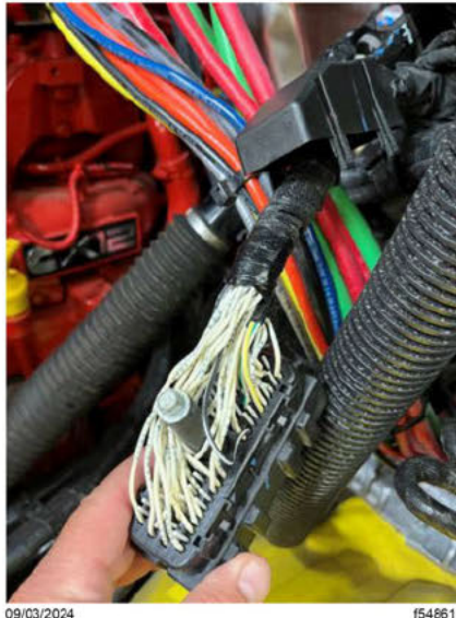
Fig. 48, Allison ECU Connector Backshell Removed
