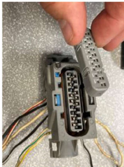
Fig. 67, Removing the Terminal Guide from the Eaton Endurant Connector
