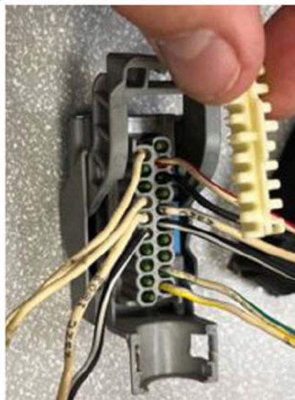
Fig. 67, Removing the Terminal Guide from the Eaton Endurant Connector
