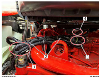
1. Fan Harness Connection to eViscous Fan 2. Fan Harness (A66-39340-000) 3. Engine Harness Connection to Fan Harness 4. Fan Controller Connector Fig. 55, eViscous Fan Harness A66-39340-000 (Installation May Vary)
