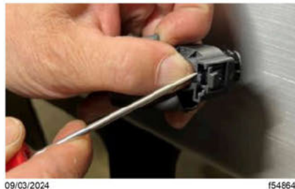
Fig. 77, Removing Outer Shell From Forward Radar Connector
