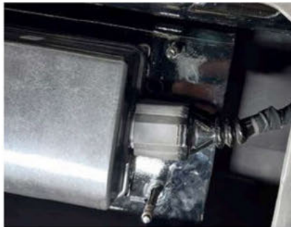
Fig. 83, Forward Radar Connector Connected to Forward Radar
