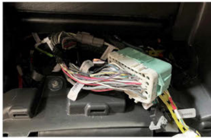
Fig. 16, Connector BHA Pulled Up into Area Behind the ICU for Access
