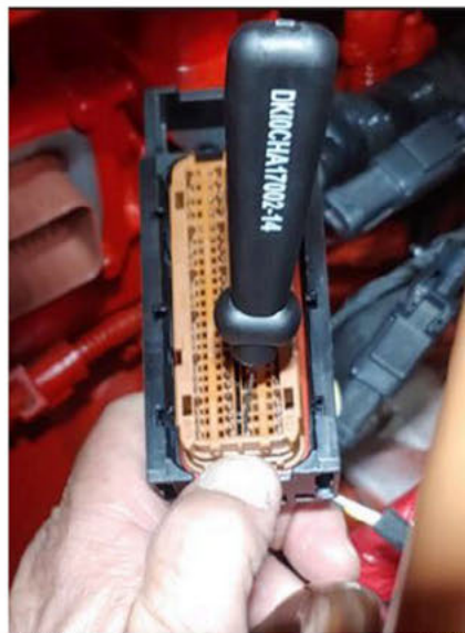
Fig. 63, Releasing and Removing J1939 Wires from the Cummins ECM Connector Using Terminal Tool DK10CHA17002-14
