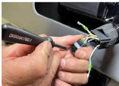
Fig. 80, Removing Wires from Forward Radar Connector Using Terminal Tool DK10CHA17002-1 to Release Terminal Tangs.
