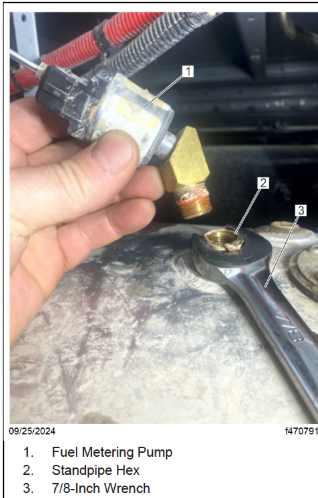
Fig. 2, Auxiliary Heater Fuel Metering Pump Removed
