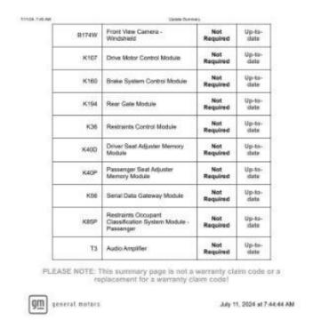
5. Once complete, the warranty claim code page will populate with details of a completed, partial, or failed programming event. Any failures will be shown at the top highlighted in red. Any successful or skipped modules will be collapsed but are viewable in a printout or clicking on an individual carrot.
