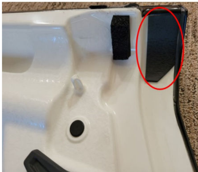
Fig. 3 Foam Pad Installed
