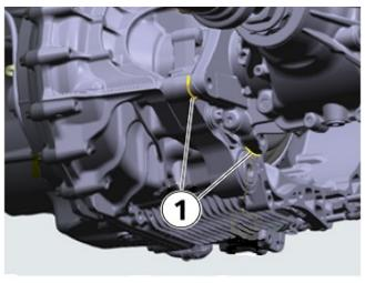
Install washers between the link and transfer case. It may be necessary to slightly push the transfer case to the side to install the washers.
