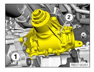
Remove the two bolts (1) on the transfer case.
