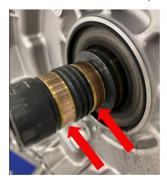
In addition, clean/wipe the slip rings (bronze rings) on the rotor, with a clean lint-free cloth (arrows).
