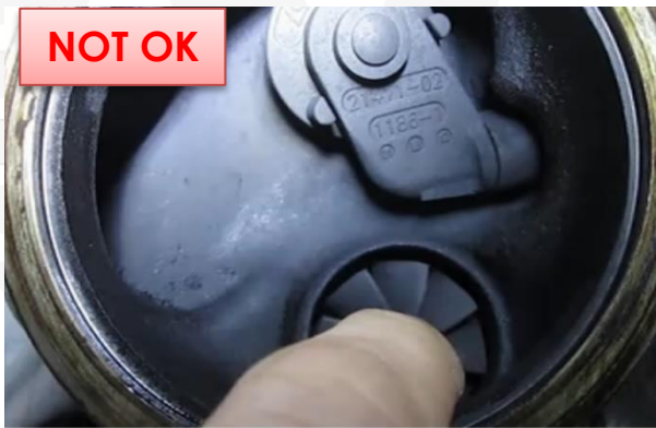
Turbine wheel excessive freeplay
