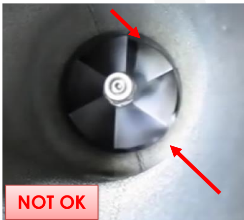
Compressor wheel excessive freeplay
