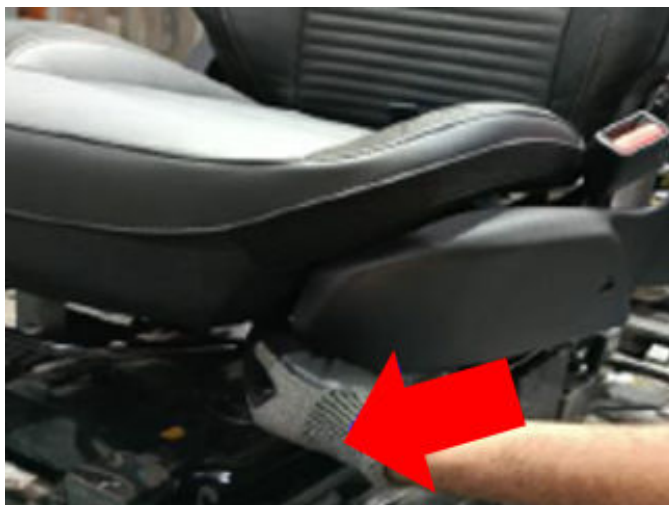
Fig. 8 Pulling Cover Off
