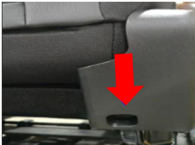
Fig. 4 Cover Fastener Location
