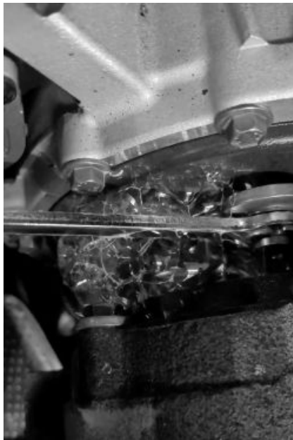
Normal turbocharger VGT shaft seal leakage.
