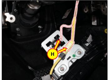
9. Locate the front driver side sunroof drain hose plug (I) underneath the crash pad and behind the Integrated Central Control Unit (ICU).
