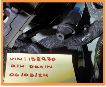
Insert the new drain hose plug (H) into the drain hole and pull on the plug by hand to ensure it is seated properly and does <u>NOT</u> come out.
