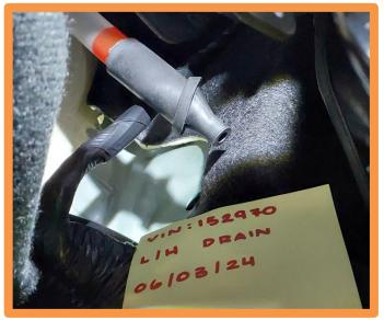
13. Insert the new drain hose plug (J) into the body and pull on the plug by hand to ensure it is seated properly and does **NOT** come out.
