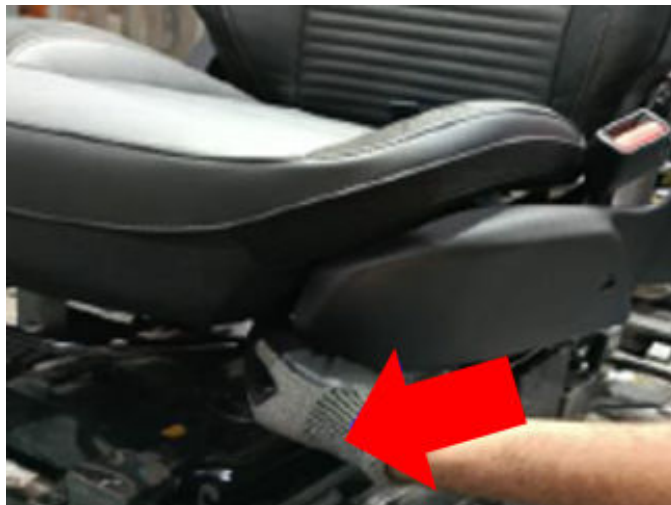
Fig. 8 Pulling Cover Off
