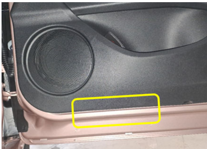
Fig. 2 Area Of Potential Leak
