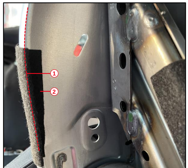
1 Edge of the Frame 2 Protector Adhered to the Inside of the Frame
