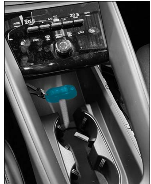
Original handheld transmitter in emergency start tray
