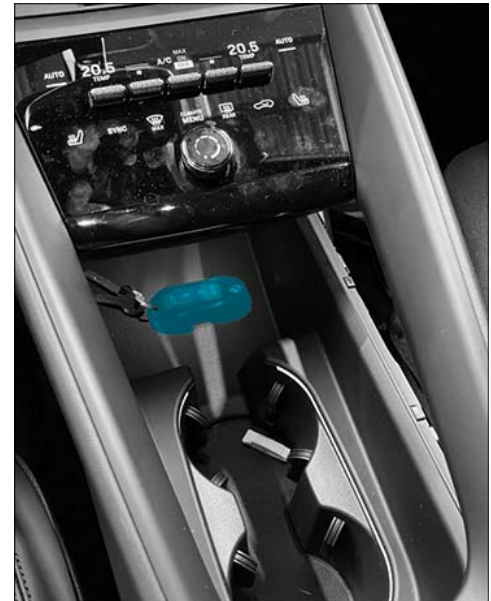
Original handheld transmitter in emergency start tray
