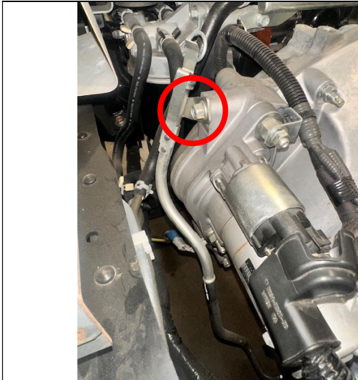
Figure 3 – Bolt Holding Oil Filler Tube
