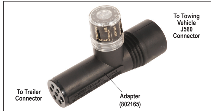
FIGURE 11 - TRDU™ TOOL AND ADAPTER
