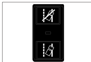
Figure 31 – LDW, HDW, & HDB Disable Switch
