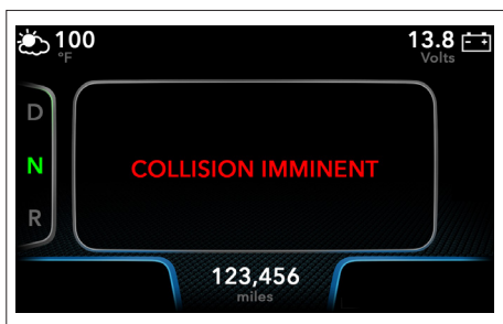
Figure 16 – AEB System Alert and Possible Autonomous Emergency Braking Applied
