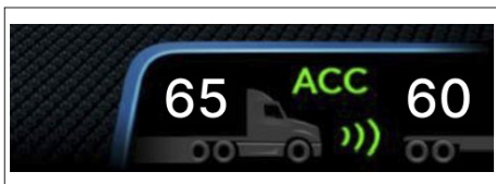
Figure 12 – Detected Forward Vehicle
