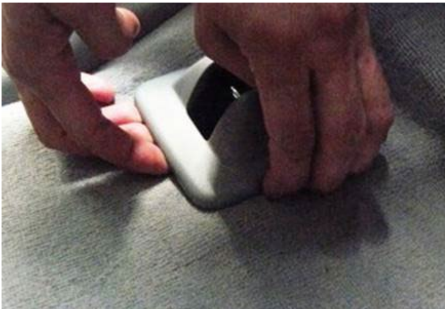
Figure 4. Remove the outer cover for the seat fastener in the floor on the door end.
