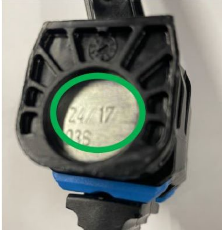
Figure 1. Replacement part with production date 24/17 (year 2024 / week 17) and component version 03S.
