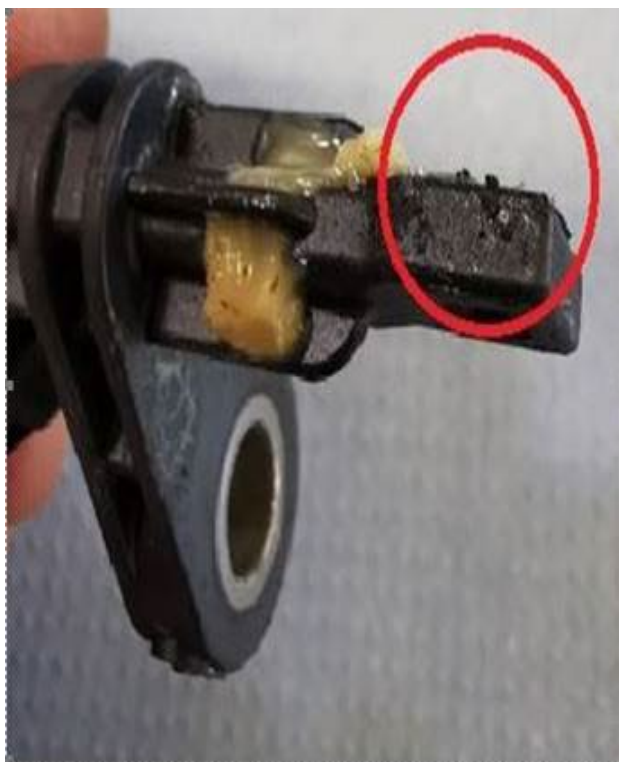
Figure 2: Metallic particles in the speed sensor.
