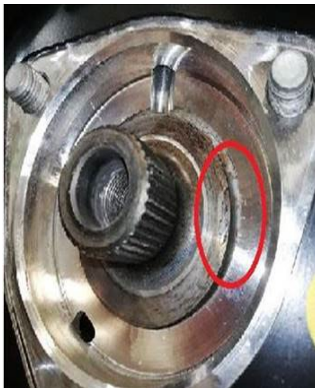
Figure 4: Metallic particles/damage in the wheel hub/bearing.
