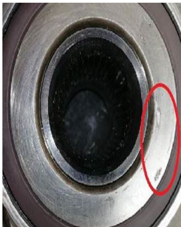
Figure 5: Metallic particles/damage in the wheel hub/bearing.
