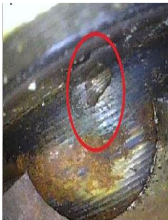
Figure 3: Metallic particles in the hub.
