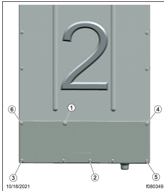
Fig. 11, Tightening Sequence for Inverter Access Cover
