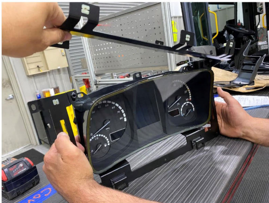
Fig. 17, Removing the ICUC from the Frame
