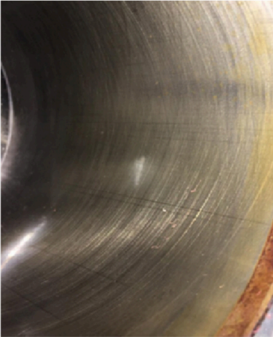
Figure 3 - Showing normal cylinder wall wear
