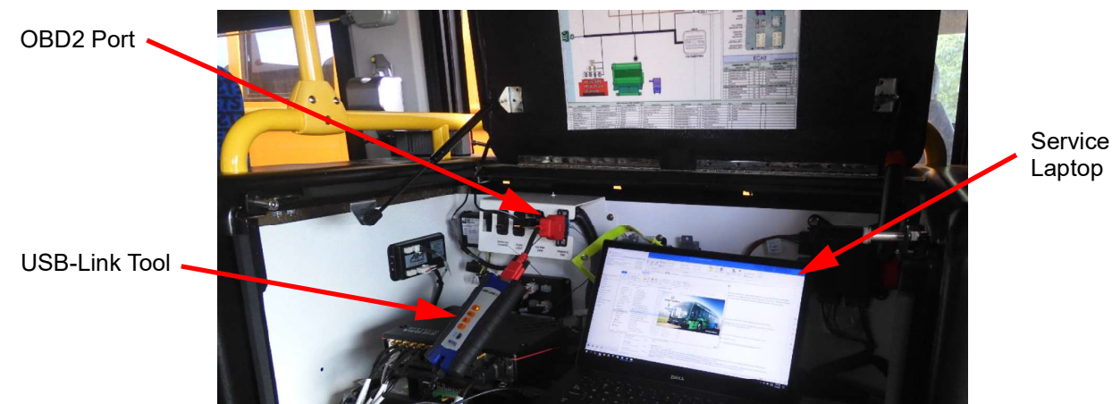
Figure 11-40. Connecting the Laptop to OBD2 Port
