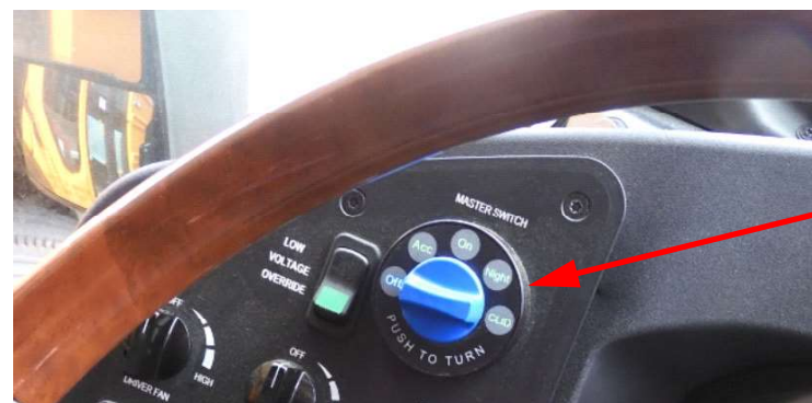
Figure 11-29. Driver Workplace Master Switch OFF
