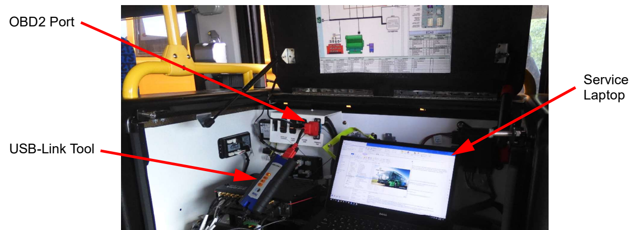
Figure 11-30. Connecting the Laptop to OBD2 Port
