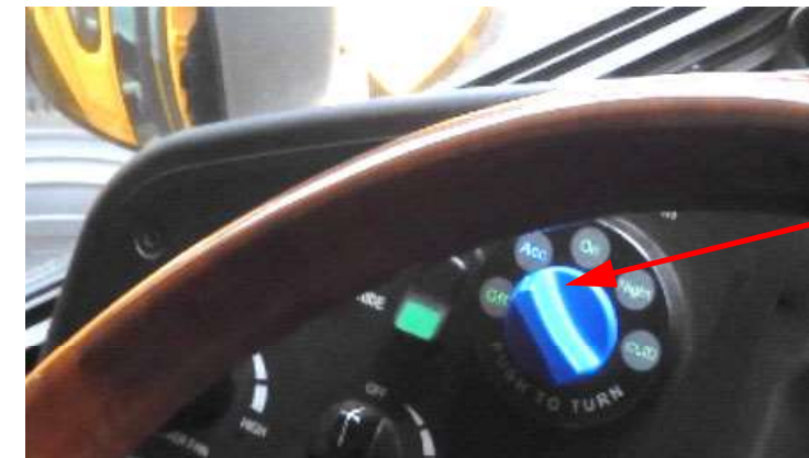
Figure 11-31. Driver Workplace Master Switch in ACC
