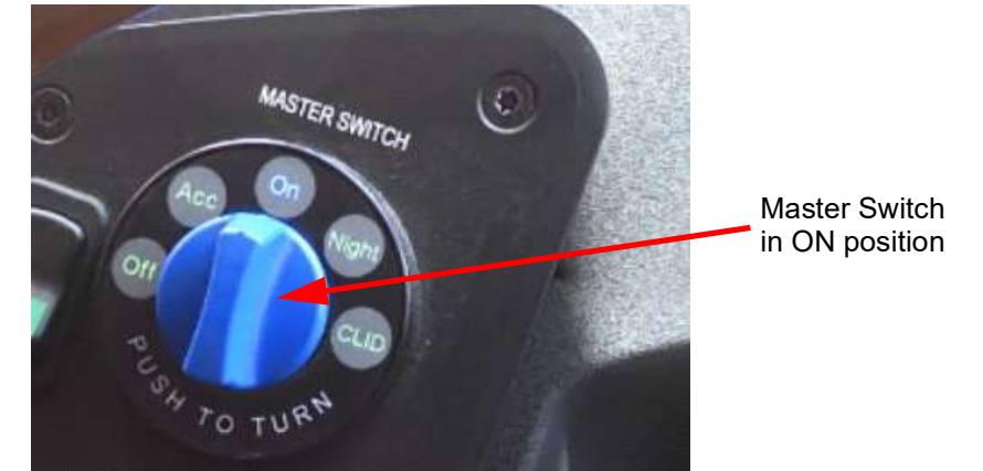
Figure 11-36. Driver Workplace Master Switch in ON
