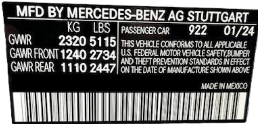
Figure 1 – B-Pillar Identification Plate
