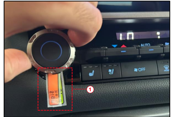
Figure 3. Aligned Flat Mounting Points
