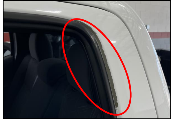
Figure 2. Paint Peeling on Inner Fender
