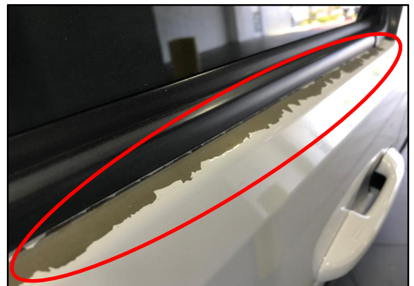
Figure 3. Paint Peeling on Door Frame
