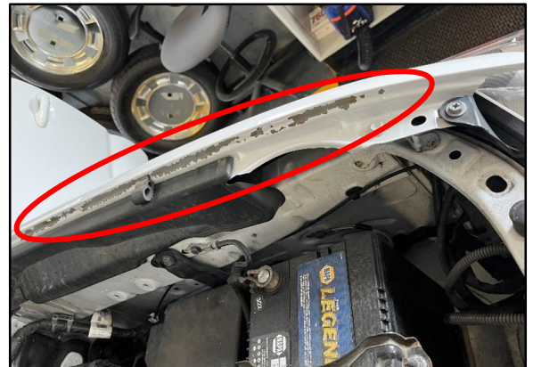
Figure 3. Paint Peeling on Door Frame
