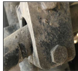
Figure 2. INCORRECT Use of Tube Clamps for Hoses
