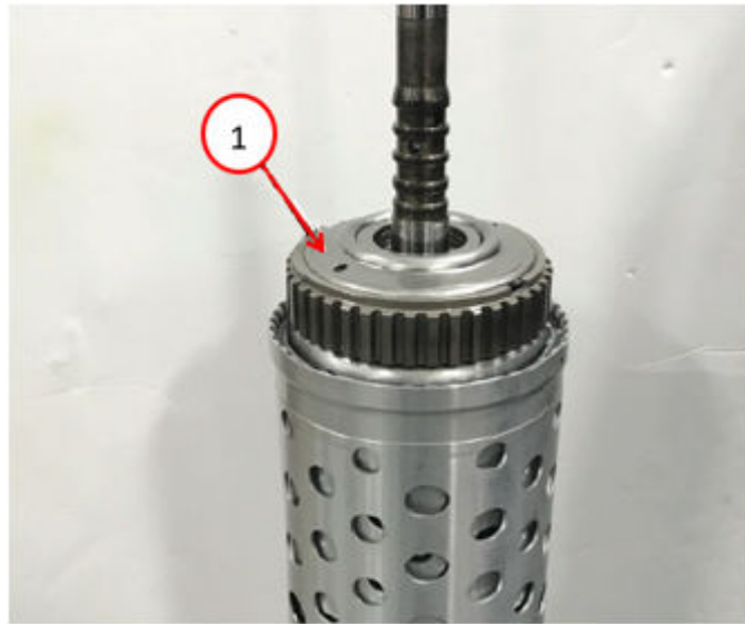
Fig. 32 P1 Annulus/B Clutch Hub Assembly
