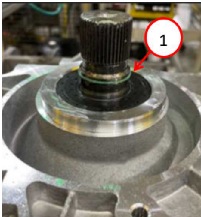
Fig. 57 WL Output Shaft Seal
