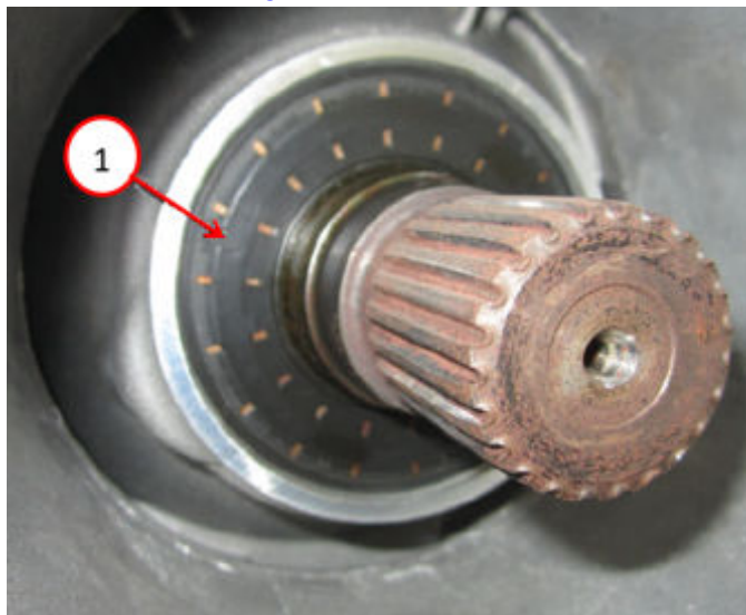
Fig. 4 Transmission Output Shaft Seal
