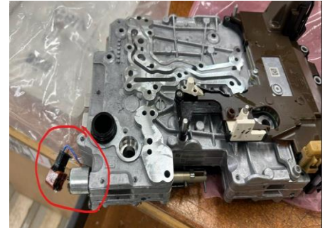
Part is broken as received at QEC due to improper part packaging.
