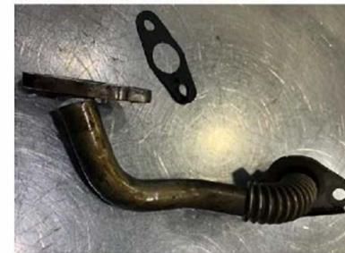
Examples of a broken turbo oil return line
