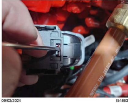
Fig. 60, Cummins ECM Connector Back Cover Removal, Disengaging the Tangs
