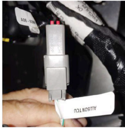
Fig. 46, End Cap Installed on Engine Harness Overlay Connector Labeled 'ALLISON TCU'
