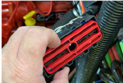
Fig. 49, Removing Terminal Guide from Allison ECU Connector
