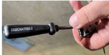
Fig. 89, Removing J1939 Wires from TPMS Connector Using Terminal Removal Tool (DK10CHA17002-2)
