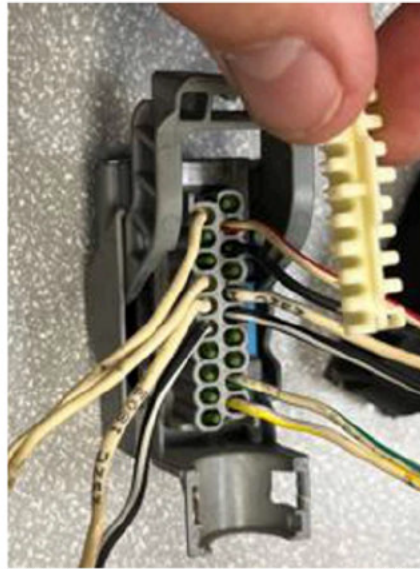
Fig. 68, Removing the Terminal Retention Clip from the Eaton Endurant Connector
