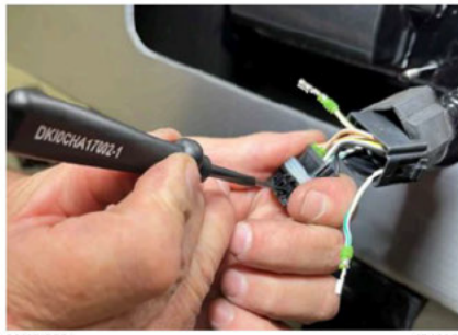
Fig. 80, Removing Wires from Forward Radar Connector Using Terminal Tool DK10CHA17002-1 to Release Terminal Tangs.
