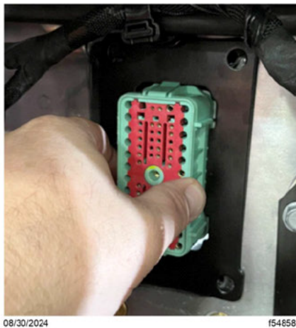
Fig. 15, Removing Bulkhead Connector BHA Mounting Plate
