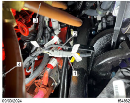
1. Jumper (A66-37414-000) 3. Bulkhead Connector BHA 2. eViscous Fan Connector 4. Engine ECM Fig. 53, Location of eViscous Fan Connector Along Engine Overlay Harness
