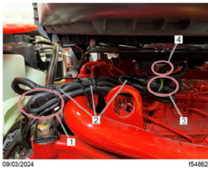
1. Fan Harness Connection to eViscous Fan 2. Fan Harness (A66-39340-000) 3. Engine Harness Connection to Fan Harness 4. Fan Controller Connector Fig. 55, eViscous Fan Harness A66-39340-000 (Installation May Vary)
