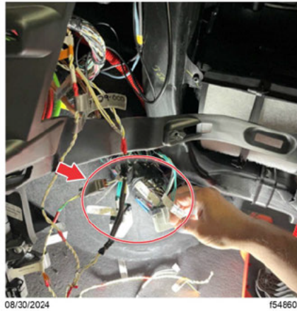
Fig. 35, Typical Location of the RP1226 Connectors that Branch Off the Main Dash Harness
