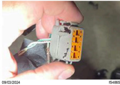
Fig. 86, TPMS Connector With Rubber Boot Slid Back Away From The Connector
