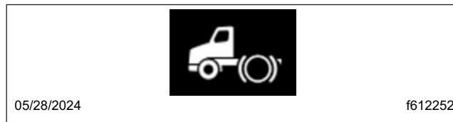
Fig. 13, Work Brake Tell-Tale on the ICU
