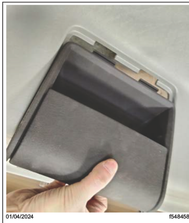
Fig. 13, Sunglasses Pocket Removal from the Overhead Console
