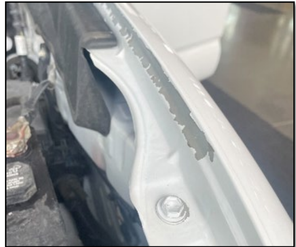
Examples of front inner fender paint peeling
