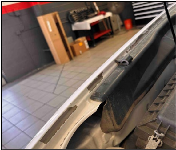
Examples of front inner fender paint peeling
