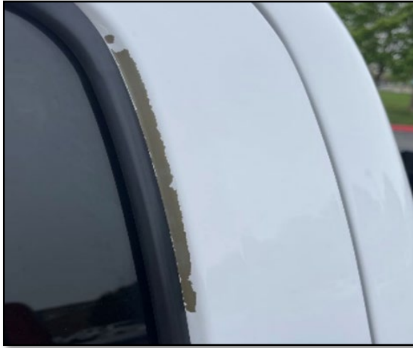
Examples of front inner fender paint peeling
