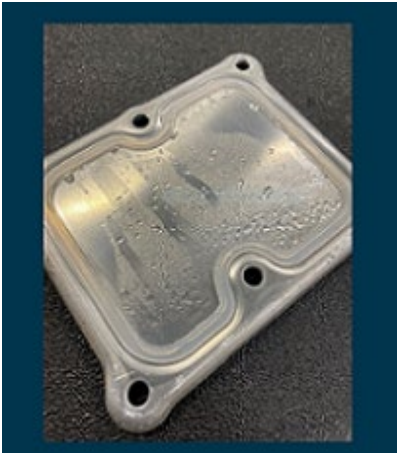
Figure 5: Condensation on high-voltage system connection cover.
