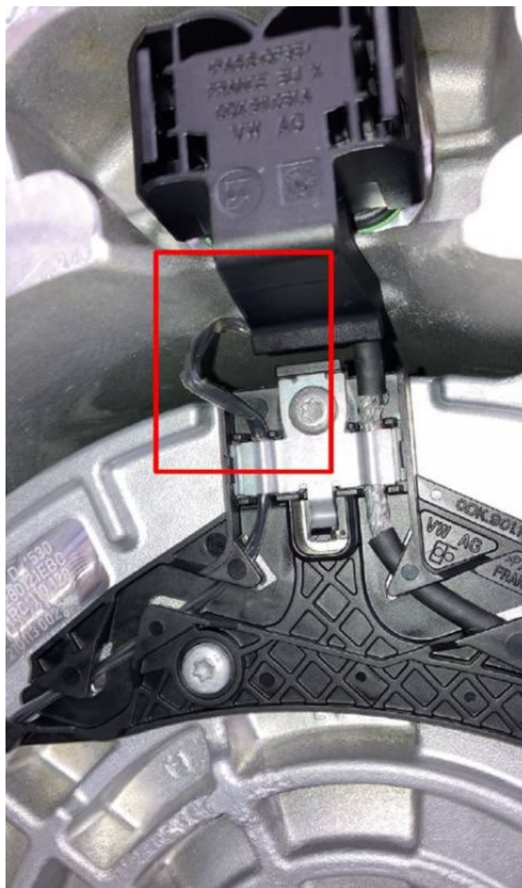
Figure 1. Wire not fitted correctly
